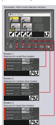
The work mode can be selected from the multi-function monitor inside the cab. Pump flow in the selected work mode can be monitored.
