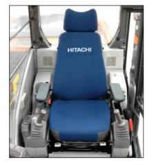
Wide adjustable armrests and a retractable seat belt are included. Short stroke levers allow for continuous operation with less fatigue. The cab is pressurized to keep out dust. Noise and vibrations are kept to a minimum due to the elastic mounts, filled with silicone oil, the cab rests on.
