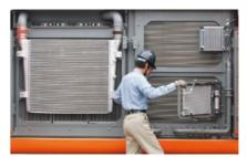
The radiator and oil cooler are separately laid out in a parallel for easy demounting, instead of the conventional in-line arrangement. This new parallel arrangement significantly helps facilitate cleaning around the radiator and oil cooler, and improving oil cooling capability. The air-conditioner condenser and fuel cooler can be opened to easily clean them and the radiator located behind.
