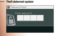
The electronic immobiliser requires the entry of an encryption code to the multifunctional monitor each time when starting the engine to prevent theft and vandalism.
